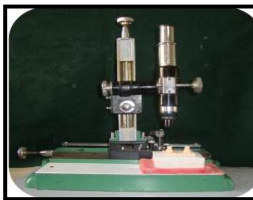
Fig.6 Travelling microscope with cast
