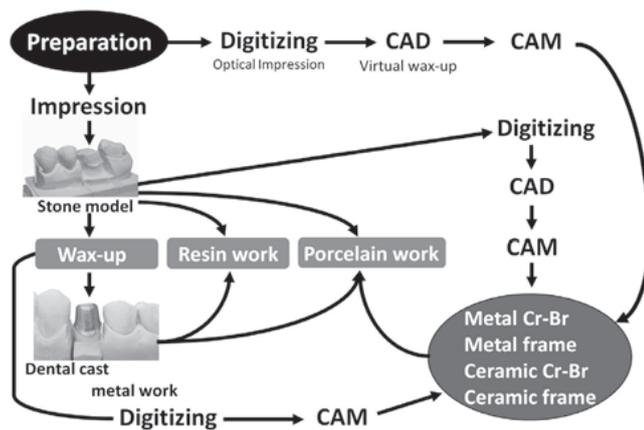
**Fig. 2 PATHWAY THE CURRENT CAD/CAM SYSTEM USES FOR FIXED PROSTHESIS FABRICATION**
