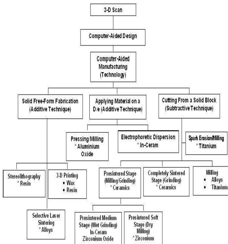
Fig.1 An overview of the CAD/CAM systems available today in dentistry.
