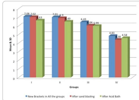
Fig 2- shear bond strength of the new brackets and after sand blasting and acid bath technique
