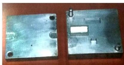
Fig: 2 Metal Die With Ceramic Sample
