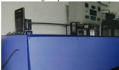
**Fig: 4 Reciprocating Sliding Wear Test Machine**
