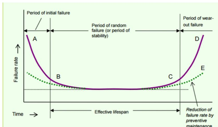
Figure 1: Failure rate curve of the same model equipment group without performing the maintenance
