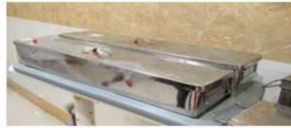
Picture 4: New Stainless-Steel Tray for Chemical Sterilization
