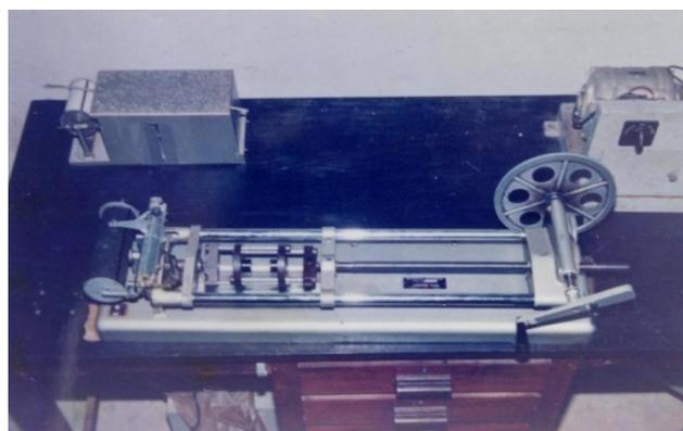
**Fig-5-Hounse Field Tensometer**
