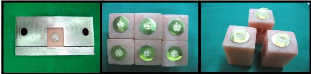
Figure 4a: mounted samples, 4b defined bond area, 4c: teflon ring for composite
