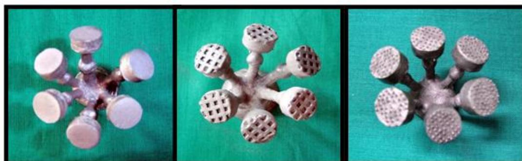
**Figure 3:** sprued resin samples
