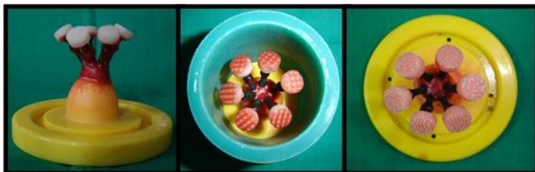
**Figure 2:** sprued resin samples
