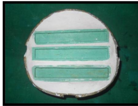
FIG- 2 FLASKING RESIN SPECIMEN
