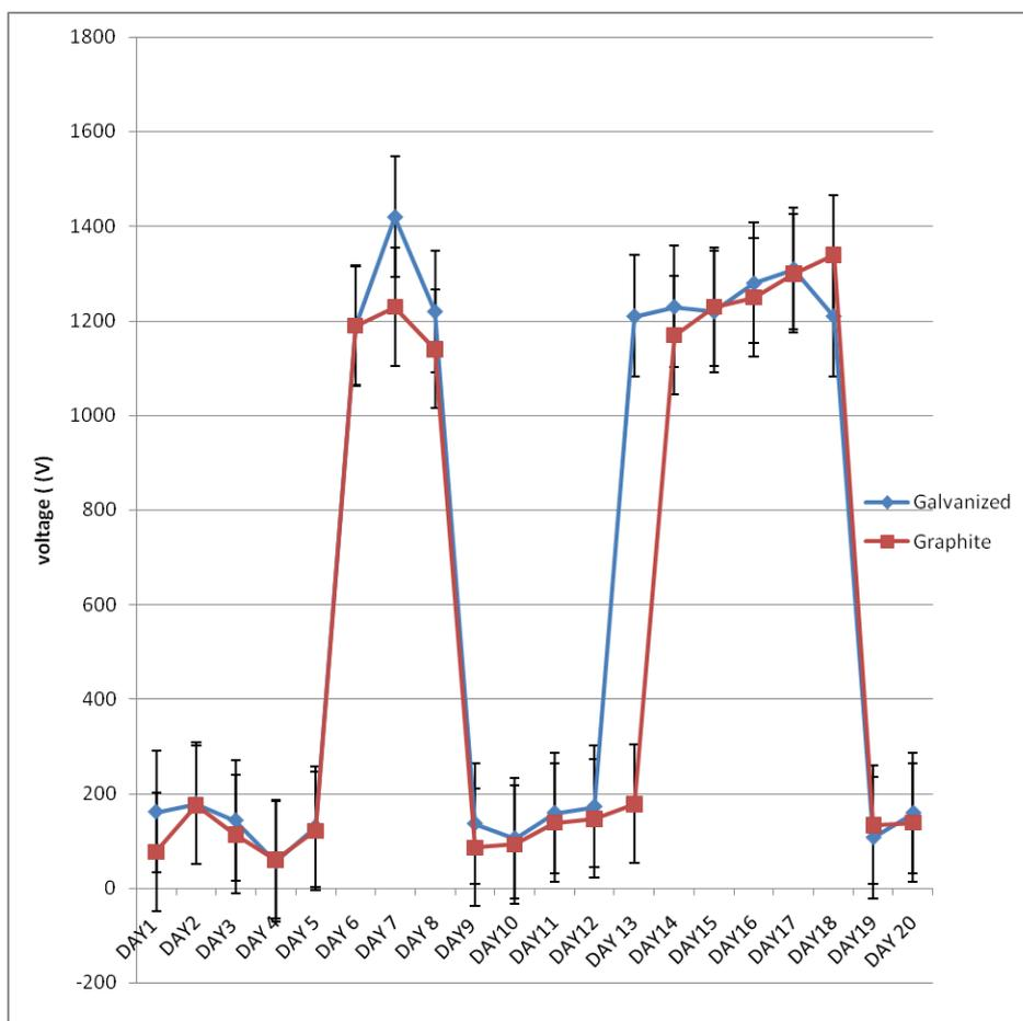
**Figure 2:** Comparison of two electrodes in MFC’s design with Nafion 117 using *Saccharomyces cerevisiae* as inoculums.
