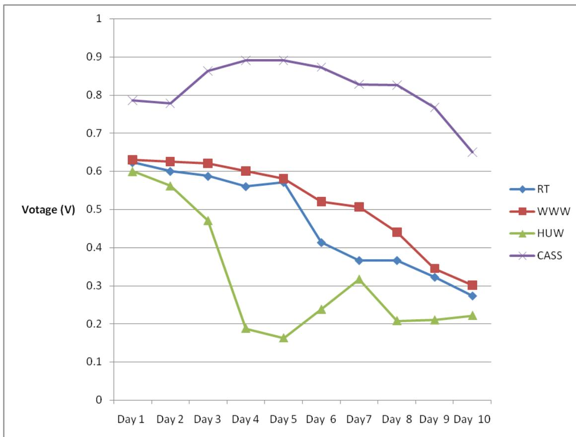
Figure 1: Screening for probable substrate from different waste using MFC Design with Salt bridge
