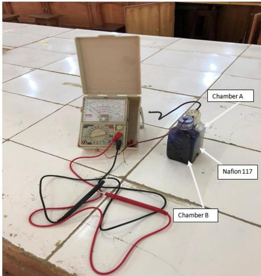
**Plate 2:** Two Chamber Microbial Fuel Cells separated by Nafion 117
