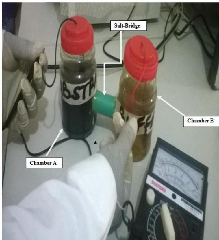
**Plate 1:** Two Chamber Microbial Fuel Cells separated by Salt-bridge
