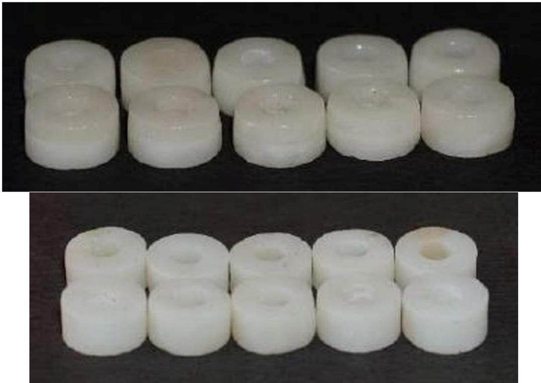
The surface of defect well of test samples from groups I &II were etched with 5% HF for 20 seconds. The samples were then rinsed with distilled water for 1 minute and air dried. (Fig. 3 & 4)
