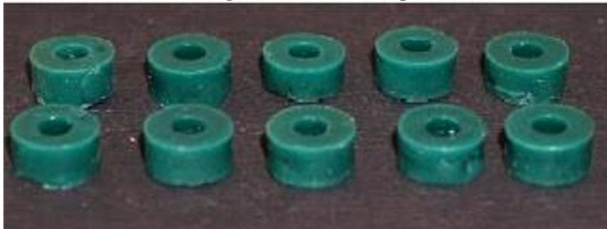
11 wax patterns for Group I were sprued and invested with phosphate bonded investment (Bellavest® SH, Germany). The burn out process was carried out at 900°C after soaking time of half an hour. Lithium Disilicate monolithic ceramic press (IPS emax press, Ivoclarvivadent, Schaan, Liechtenstein) was carried out. Divesting was done using glass beads followed by ultrasonic cleaning with 1% HF acid. Each sample was finished with water emery paper of 220, 320 and 400 grit sizes, respectively.
