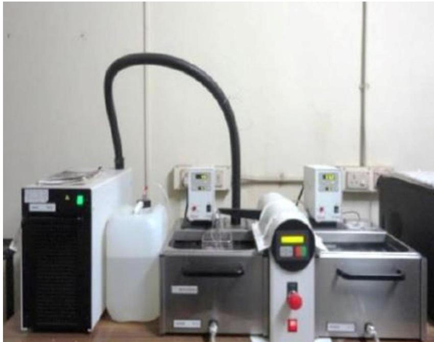
**Fig 11- Thermocycling of the test samples**
