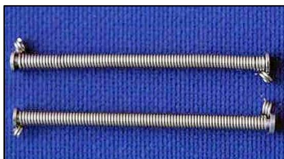
**Fig 18.Amoric torsion coils**
