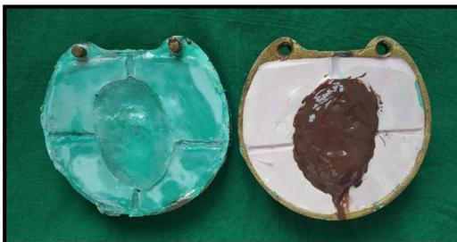
Figure 13: Packing of silicone in dewaxed mould
