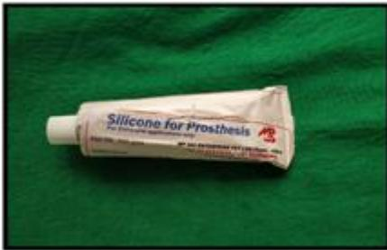
Figure 11: RTV Silicone material
