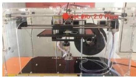
Figure 2: CoLiDo 2.0 plus 3D printer used for fabricating of special tray to duplicate master die
