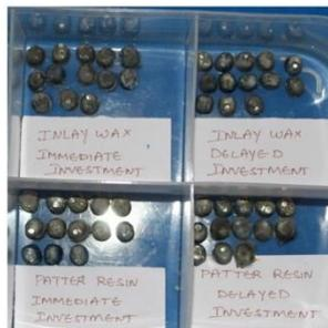
Figure 4: Metal Copings fabricated using inlay wax and auto polymerized pattern resins
