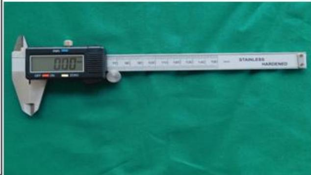
Fig 4 -sliding digital caliper
