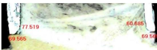
Fig.10 Measuring marginal adaption of Copings casted from milled resin patterns (group II) under stereomicroscope
