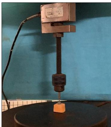
Fig. 7. Cementation of coping on respective die with 50N pressure with UTM
