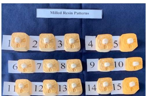
Fig. 6. Milled resin patterns
