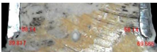
Fig.9 Measuring marginal adaption of Copings casted from 3D Printed resin patterns (group I) under stereomicroscope
