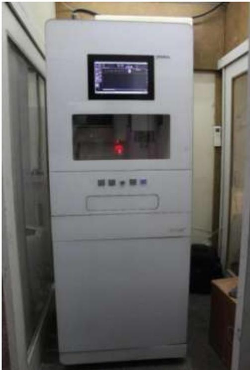
Fig 3: ZUBLER DC5 Milling Machine
