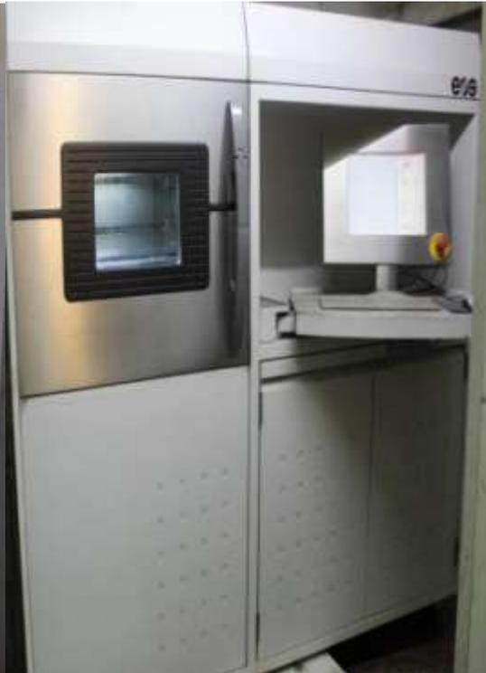
Fig 4: Direct Metal Laser Sintering EOS Germany Machine
