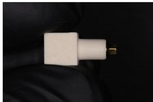
For each group, the resulting object was detached from the disc and measured using a digital caliper. The cuboid was attached to its respective ti-base and the complex was repositioned to the 3D printed model on the implant analog. It was screwed to a tightening torque of 25 N. The model was rescanned using the extra-oral scanner and a total of 10 STL files were created for each group.
