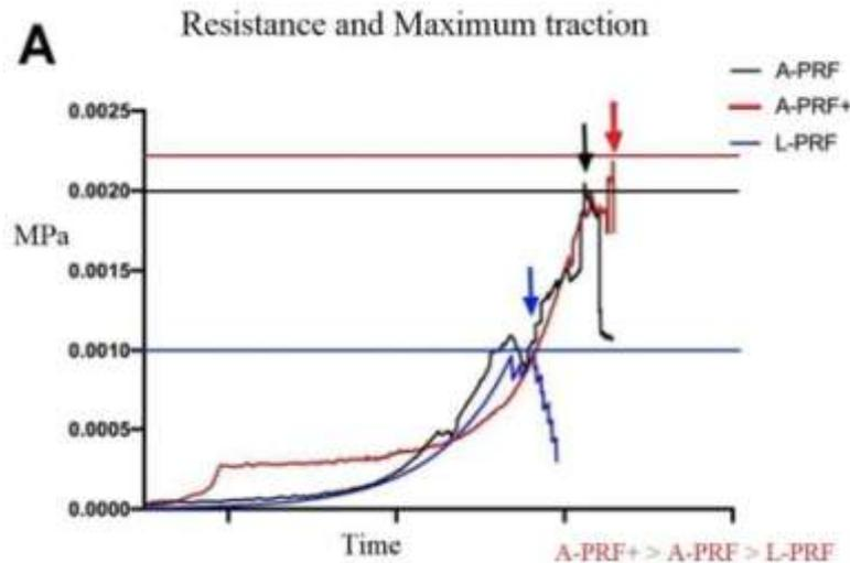
Fig.3 Resistance and maximum traction of the PRF
