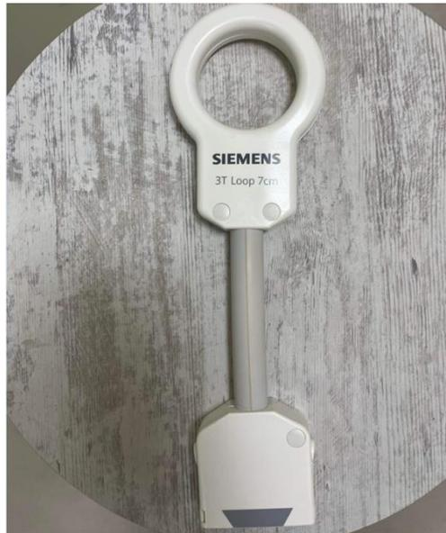
**Fig. 1. Specialized eye socket coil (loop coil)**
