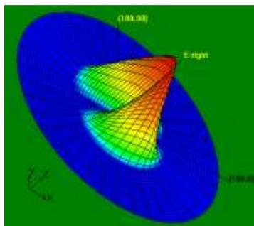
Figure 7: E-Plane (3D View) Radiation Pattern for slotted antenna at 9.54 GHz
