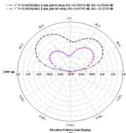
Figure 10: H-Plane (2D View) Radiation Pattern for slotted antenna at 12.90 GHz
