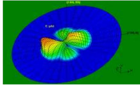
Figure 12: H-Plane (3D) Radiation Pattern for slotted antenna at 12.90 GHz
