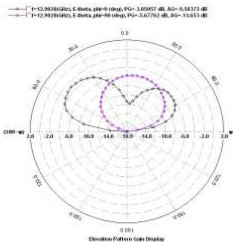
Figure 9: E-Plane (2D View) Radiation Pattern for slotted antenna at 12.90 GHz
