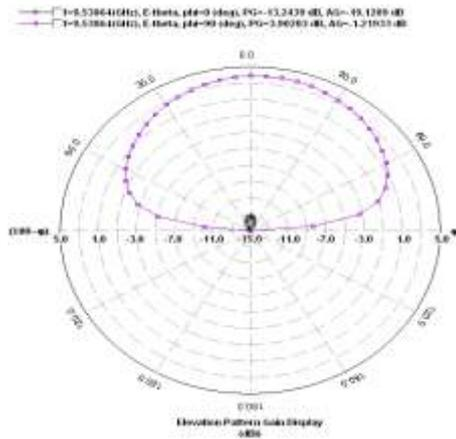
Figure 5: E-Plane (2D View) Radiation Pattern for slotted Antenna at 9.54 GHz
