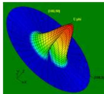
Figure 8: H-Plane (3D View) Radiation Pattern for slotted antenna at 9.54 GHz
