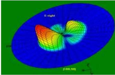
Figure 11: E-Plane (3D View) Radiation Pattern for slotted antenna at 12.90 GHz
