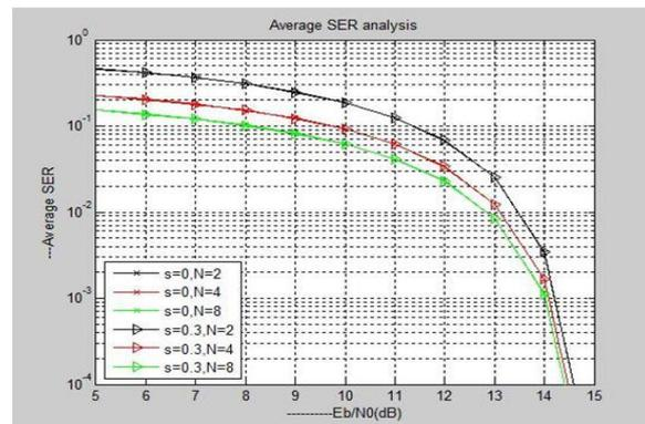
Fig. 4 The average SER as a function of SNR Proposed MSDD receiver with QDDPSK  $\psi=0.3$  & selected values of  $N$ .
