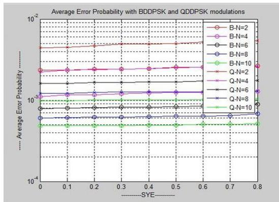
Fig.2 The average error probability of the proposed for the MSDD as a function of  $\psi$  with BDDPSK & QDDPSK modulation, modulation for  $\text{SNR}=10\text{dB}$  &  $N=2,4,6,8$  and  $10$ .
