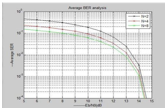
Fig.3 The average BER as a function of SNR for the proposed receiver and the autocorrelation demodulator detection with BDDOSK modulation,  $\psi=0.3$ , and selected values of  $N$ .
