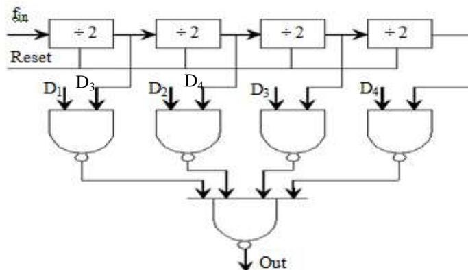
Fig. 10. Block diagram of a swallow counter.
