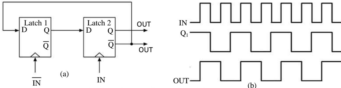
Fig. 5. (a) Divide by 2 prescaler and (b) timing diagram.
