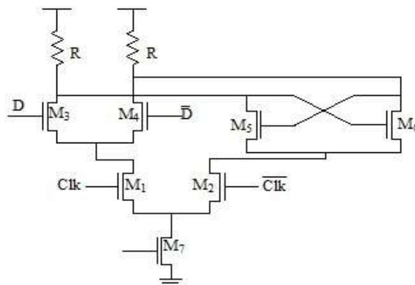
Fig. 2. Schematic of an SCL D latch.
