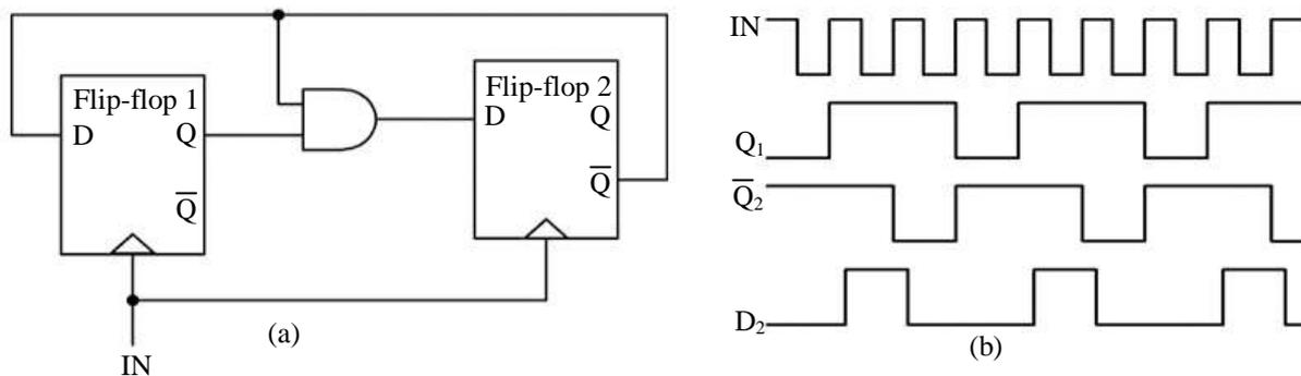
Fig. 6. (a) Divide by 3 prescaler and (b) timing diagram.
