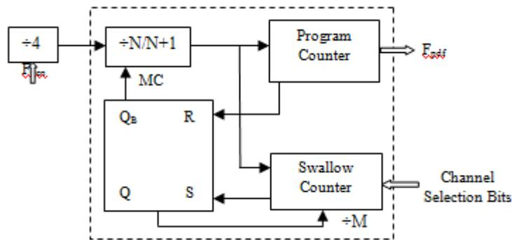
Fig. 4. Programmable Frequency Divider.
