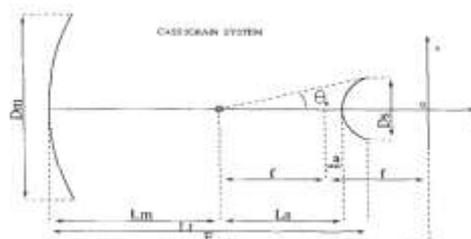
Fig1. Geometry of the Cassegrain Antenna
