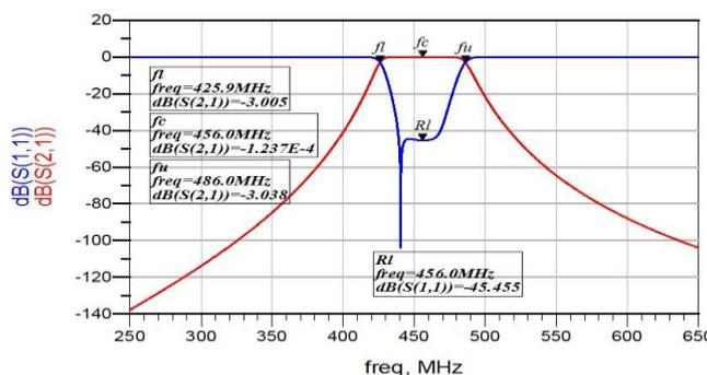
Figure 4. S-Parameters result from ADS 2011
