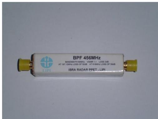
Figure 7. Photograph of bandpass filter with package
