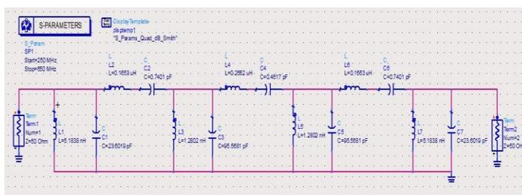
Figure 3. Schematic of bandpass filter
