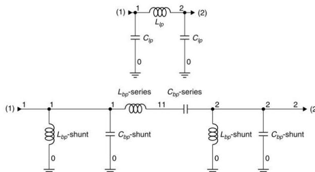
Figure 1. Bandpass filter prototype starting with low pass filter
