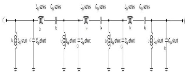
Figure 2. Bandpass filter with  $N=7$
