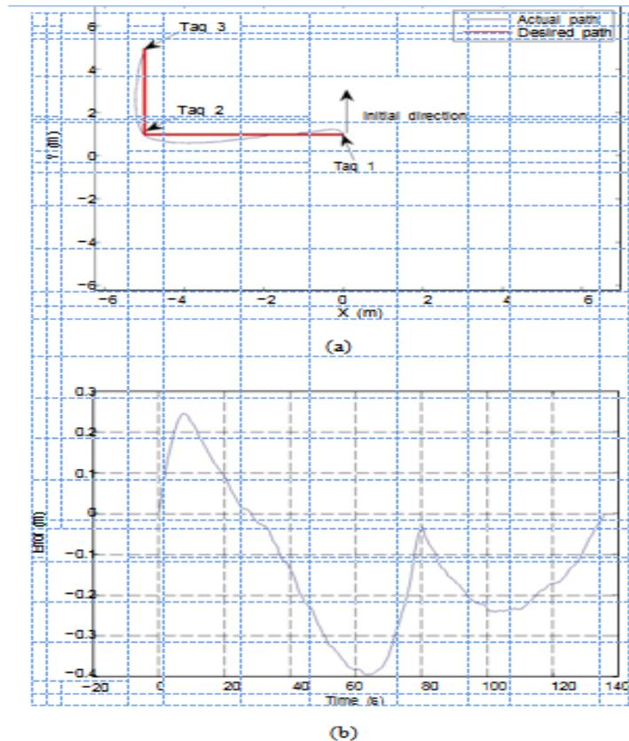
The proposed algorithm is very modular as it can be easily implemented on virtually any type of robotic systems and working environments. It is computationally inexpensive as it is free of any visual data processing
