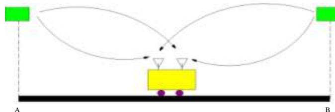
Figure 2. High-level system configuration with two RFID tags.
