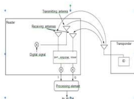
Figure 1. RFID system setup to compute the phase difference.
