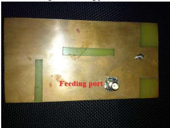
Figure 6: Hardware image (Ground plane)
