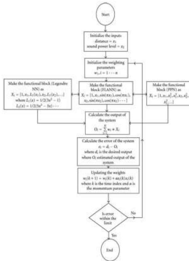
Figure 3: Systematic algorithm of functional based neural network
