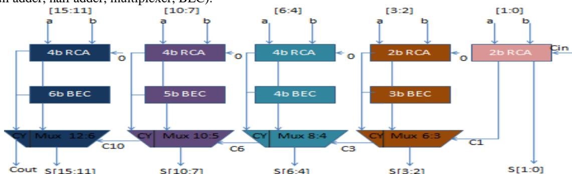
Fig.4.Modified Carry Select Adder
