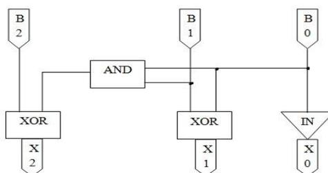
Fig.1 3-Bit Binary to Excess-1 Converter
