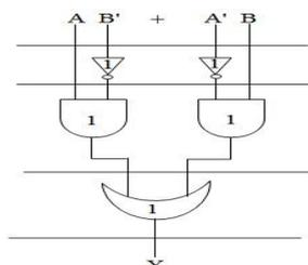
Fig.2 Delay and Area Evaluation of an XOR Gate
