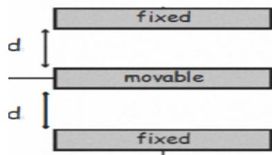
Fig. Equivalent model of capacitive accelerometer
