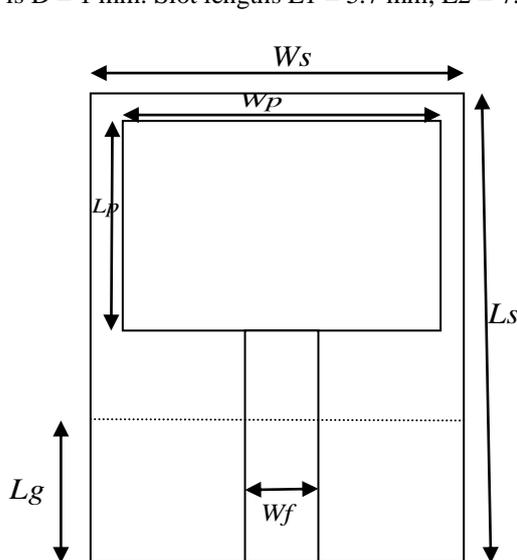
Fig1: RMP antenna design
