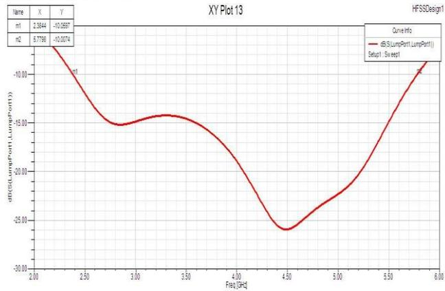
Fig4: Return loss of RMPA with slots
