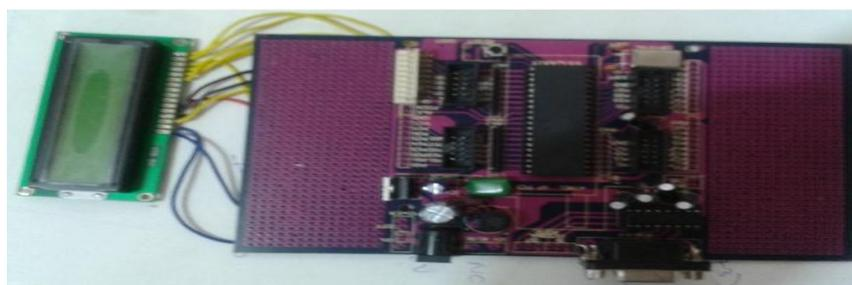
Fig. 8: Microcontroller-89c52 Board
