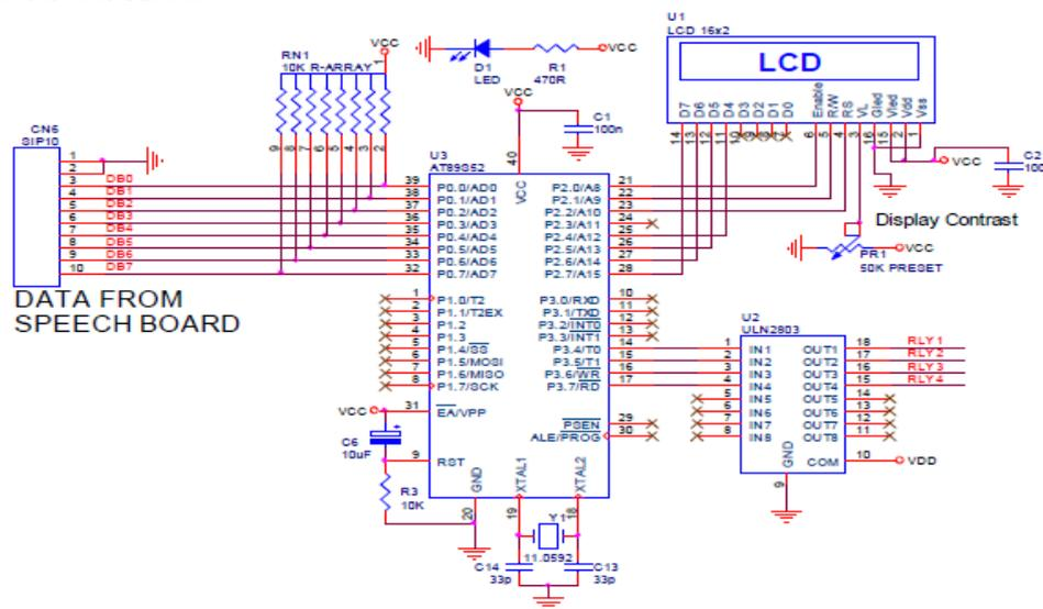
Fig. 7: Microcontroller Module.
