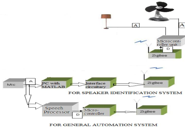
Fig.1: Functional Block Diagram of Automation system for Speaker Identification
