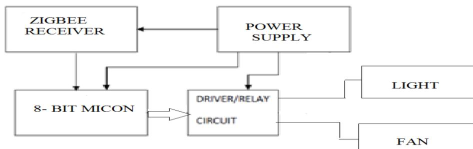
Fig. 3: Receiver section.
