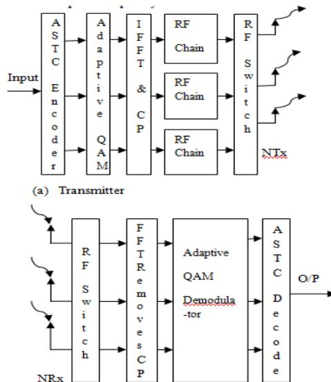
Fig 1: Block Diagram of MIMO-OFDM system (a) Transmitter and (b) Receiver
