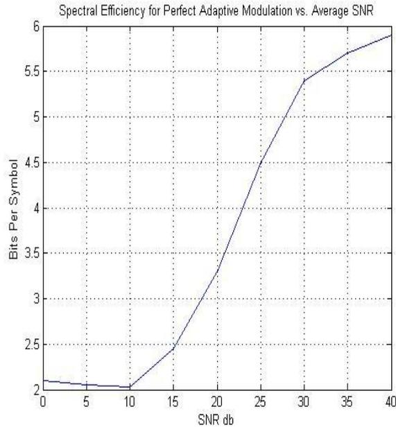
Fig. 5 Spectral Efficiency for Perfect Adaptive Modulation vs. Average SNR for a Rayleigh Channel
