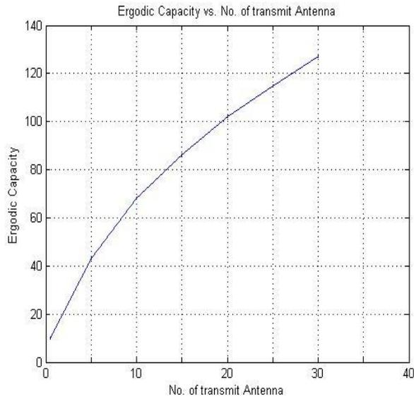
Fig. 3: Ergodic capacity versus no. of transmit antenna
