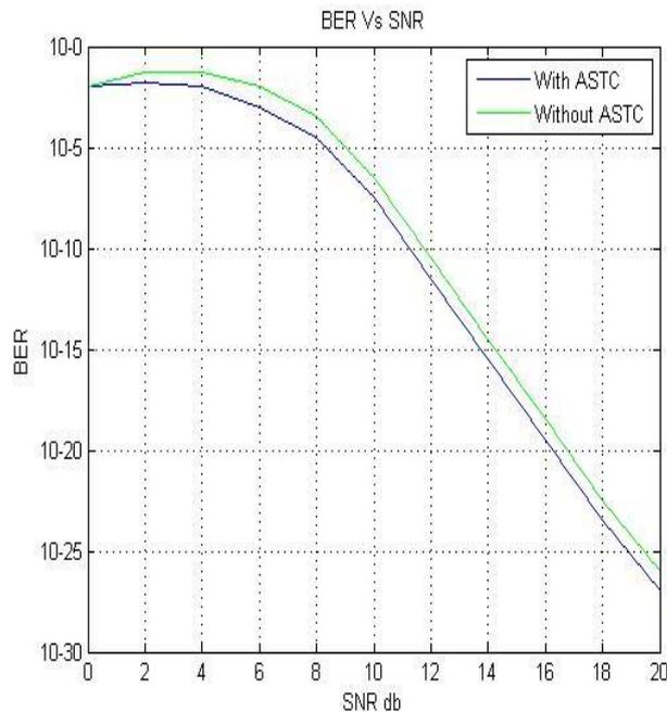
Fig. 6 System performance by using ASTC encoder w.r.t. SNR vs BER
