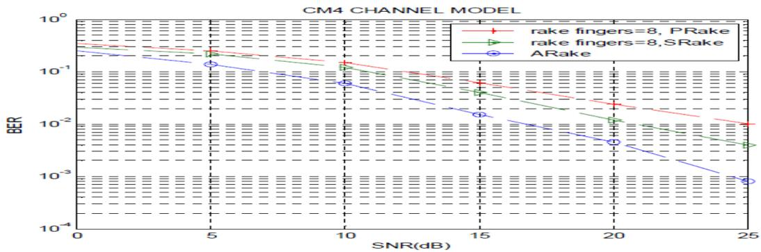
Fig. 4 BER performance of Rake receiver for CM4 channel model
