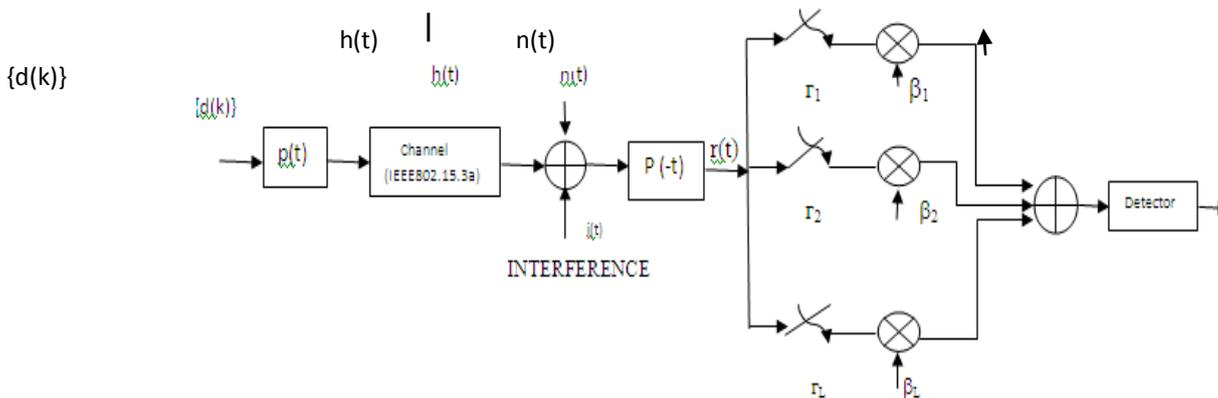
**Fig.2 UWB Rake receiver model in presence of NBI**
