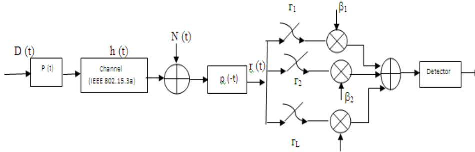
Fig.1 UWB Rake receiver model in presence of NBI
