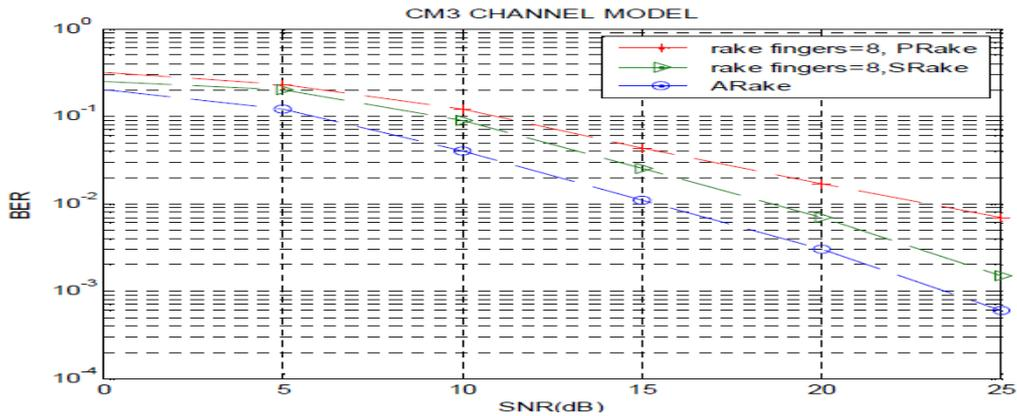
Fig.3 BER performance of Rake receiver for CM3 channel model
