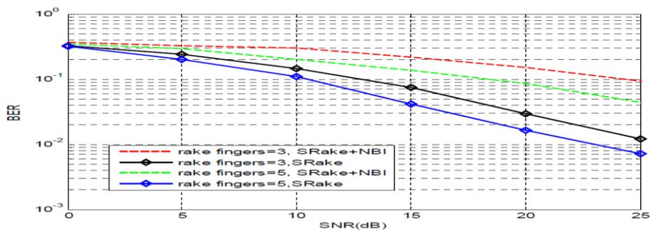
Fig. 5 Performance of SRake receiver for CM3 channel model
