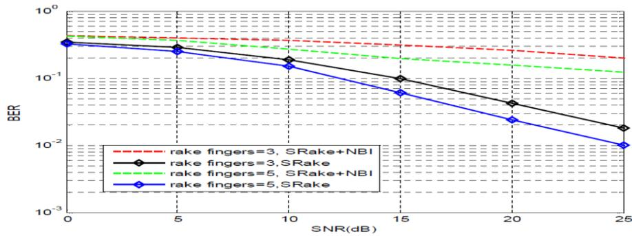
Fig. 6 Performance of SRake Receiver for CM4 channel model
