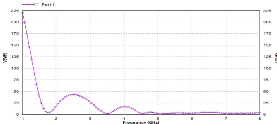
(Fig-(3.2): VSWR curve of base shaped antenna)
