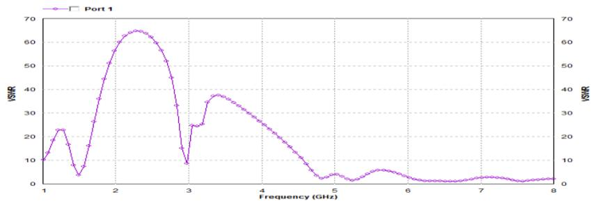
(Fig-(3.8): VSWR curve of 1<sup>st</sup> iteration)
