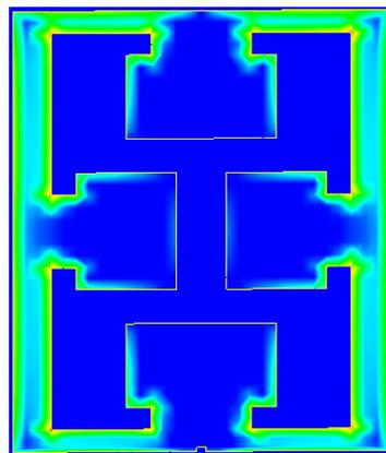
Fig-(3.11) current distribution of final patch shape
