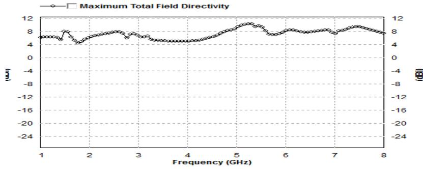
(Fig-(3.10): directivity Vs Frequency graph 1<sup>st</sup> iteration)
