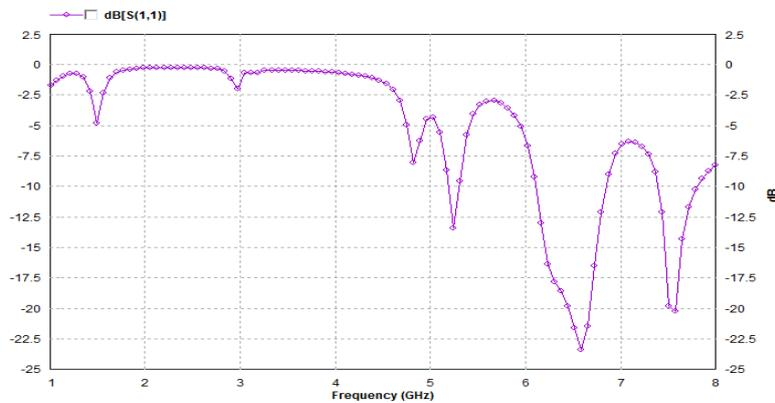
(Fig-(3.7) Return loss curve of 1 iteration)
