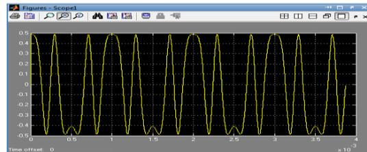
Fig:9. Time domain analysis of Quadrature component
