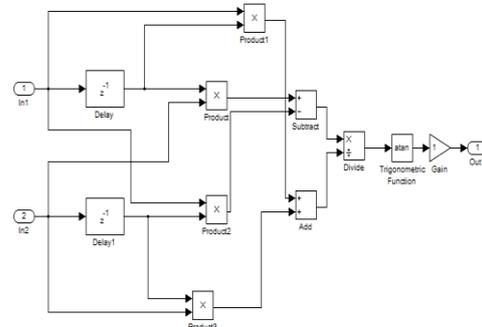
Fig:7. FM Mixed Dem odualtor Algorithm.
