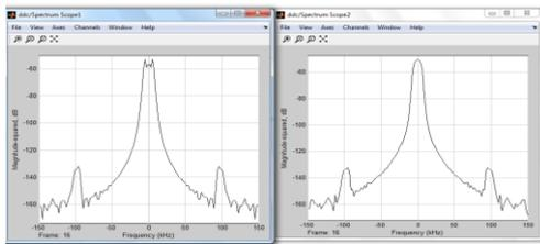
Fig:8. Frequency domain analysis of Inphase and Quadrature phase of DDC
