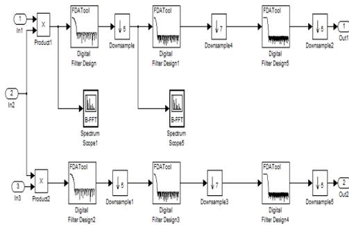
Fig:4. DDC with different stages to form a down sample factor of 175.
