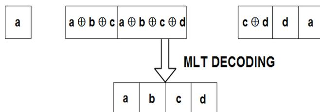
Fig. 2 Modified Luby Transform (MLT) Decoding
