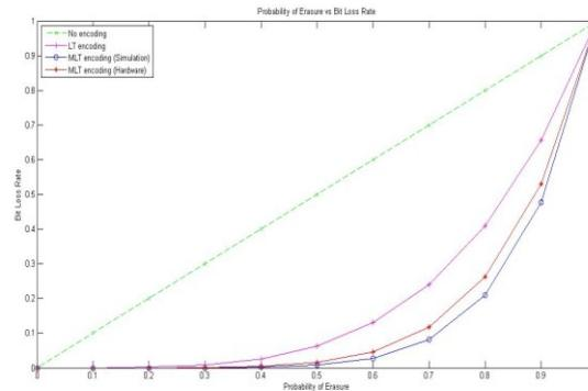
Fig. 3. Performance Analysis using Probability of Erasure vs Bit Loss Rate graph – (a) No encoding (b) LT encoding (c) MLT encoding (Simulation Results) (d) MLT encoding (Hardware Implementation Results)
