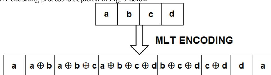
Fig. 1 Modified Luby Transform (MLT) Encoding
