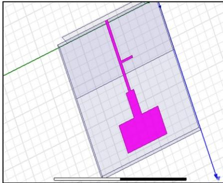
Figure 2: Design of the Patch Antenna on HFSS
