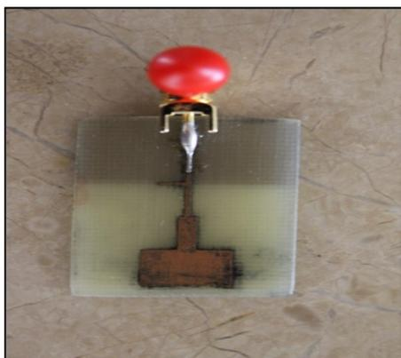
Figure 6: PCB Design of a T shaped Antenna
