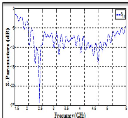
Figure 7: S Parameters and Frequency on VNA
