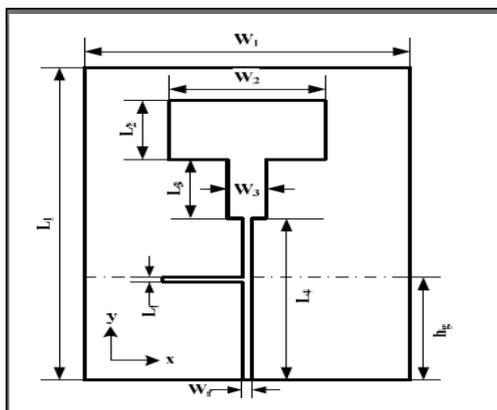
Figure 1: Design of a T-Shaped Antenna
