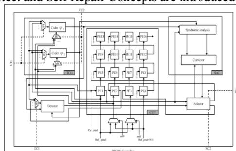
Fig1: Block Diagram of Proposed MECA BISDC.
