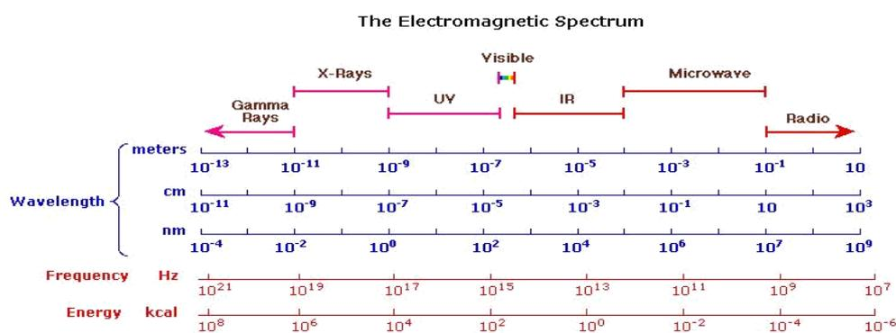
Figure 3. The full range of Electromagnetic spectrum
