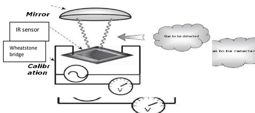
Figure 5. Sensing Mechanism
