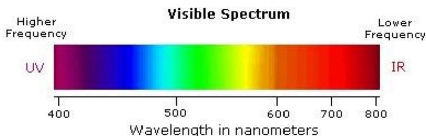
Figure 2. Electromagnetic spectrum
