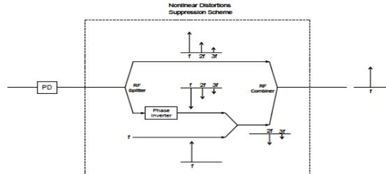
Fig. 3. Functional diagram of the nonlinear distortions suppression scheme.
