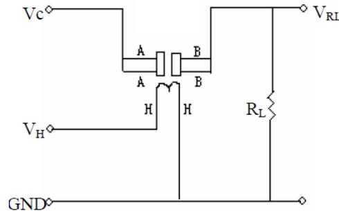
Figure 6: Test circuit of sensor
