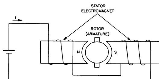
Figure 8: DC motor with electromagnet as stator
