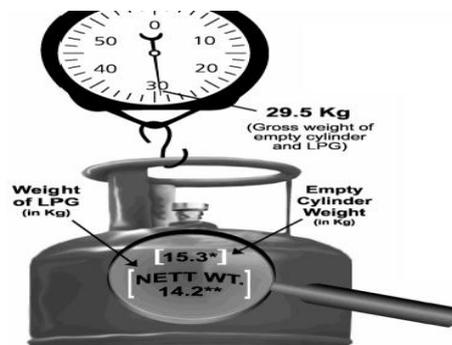
Figure 7: Weight of normal LPG gas cylinder:
