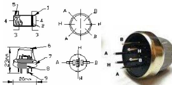
Figure 5: The structure and configuration of MQ6 gas sensor
