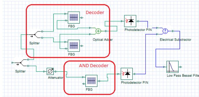
Figure 1 Modified-AND subtraction detection.
