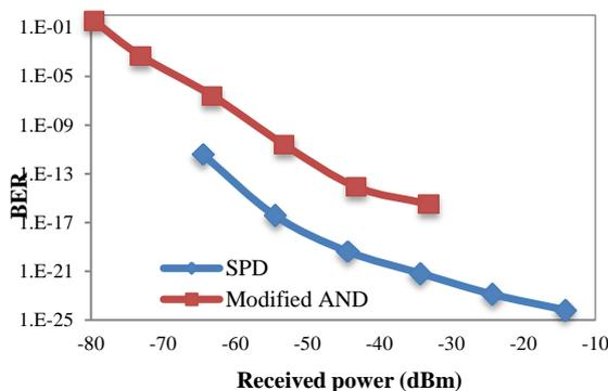
Figure 6 BER versus the received power in different detection techniques.
