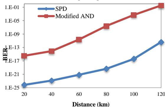
Figure 4 BER against fiber length using different detection techniques.
