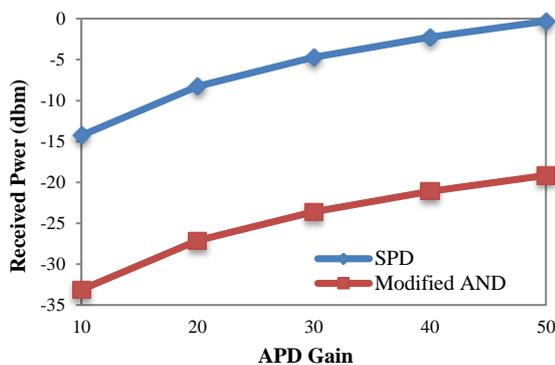
Fig. 7 Received power against APD gain in different detection techniques.
