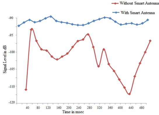
Fig 7. Minimization of the effects of Fading
