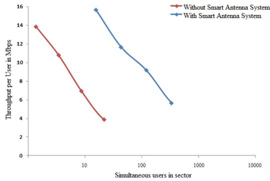
Fig 8. Improvement of throughput in the proposed uplinking
