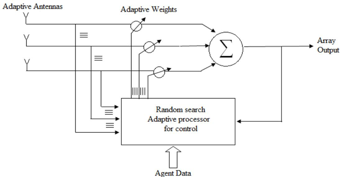
Fig 4. Proposed System – Adaptive Smart Antenna Configuration
