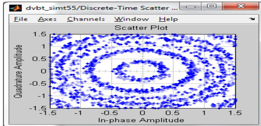
**Figure 1.5 Signal Constellation using delay vector of  $[0 \ 1e-9]$**
