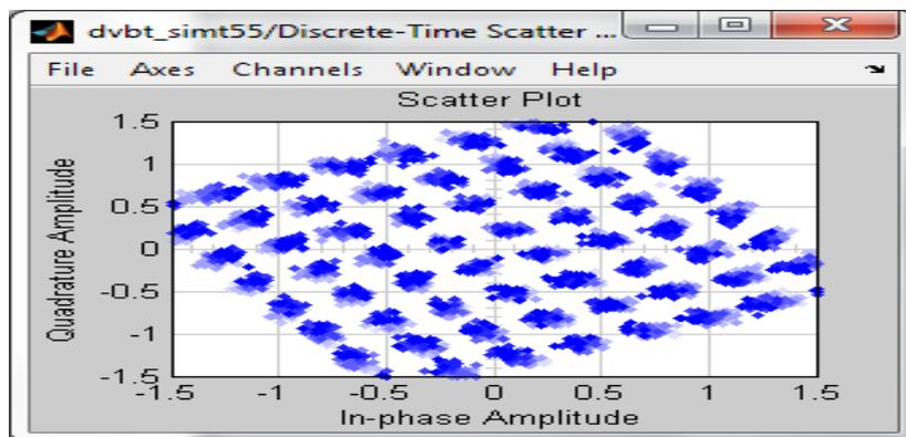
**Figure 1.4 Signal Constellation received with fading at 50Hz.**
