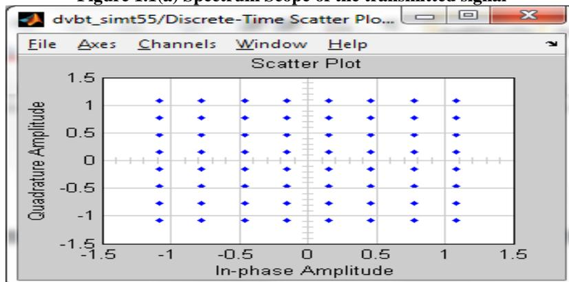
Figure 1.1(b) Signal Constellation of Transmitted signal
