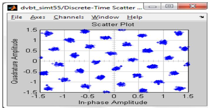
**Figure 1.3 Signal Constellation received with less noise**
