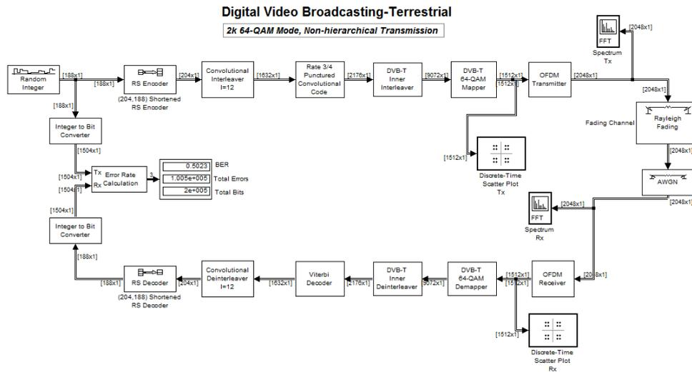
Figure 1.0 DVB-T Block Diagram Using SIMUINK
