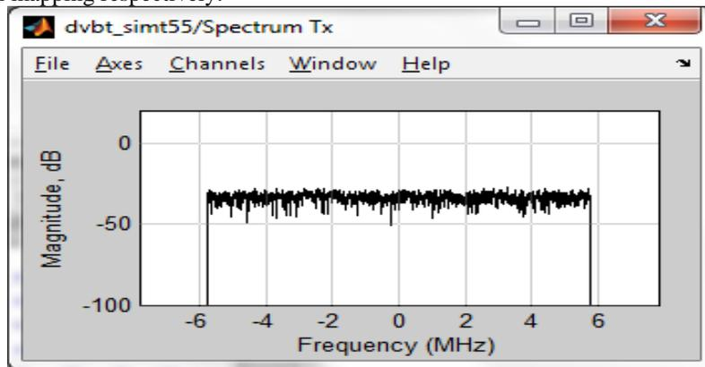
Figure 1.1(a) Spectrum Scope of the transmitted signal
