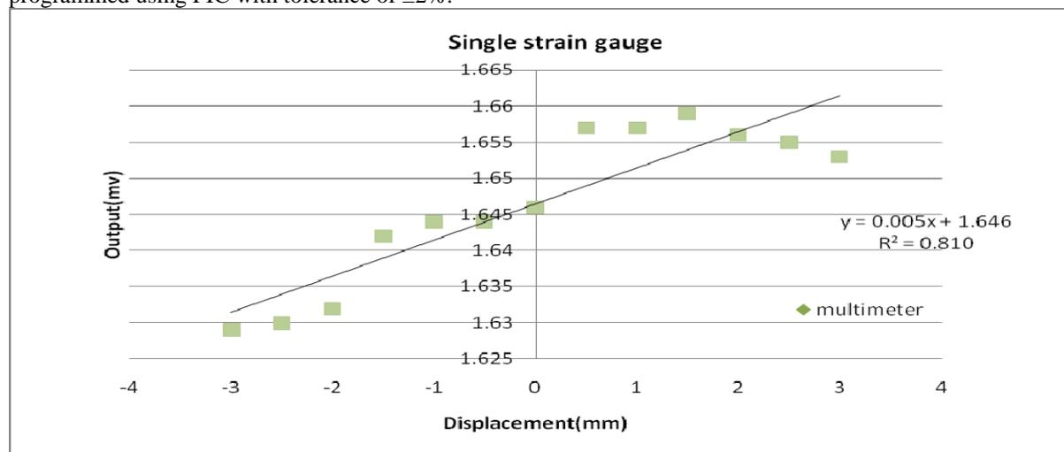
Figure 2.4: Single strain gauge
