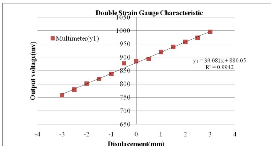
Figure 2.5: Double strain gauge
