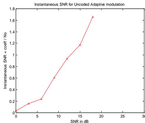
Figure 3. Instantaneous SNR of Uncoded AOFDM with BPSK,QPSK,QAM
