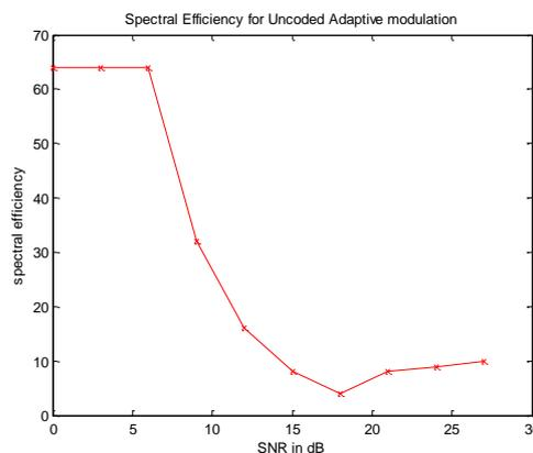
Figure 5. Spectral efficiency of Uncoded AOFDM with BPSK,QPSK,QAM
