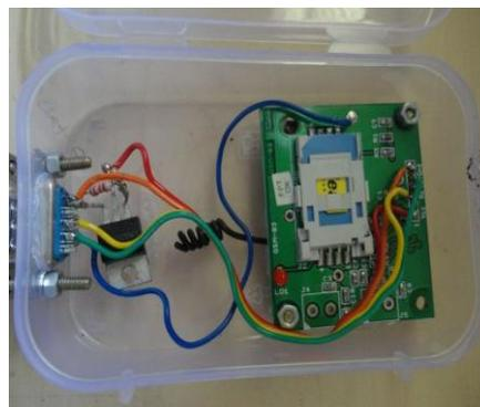
Fig 2.3. GSM Module
