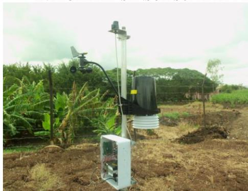
Figure 3.1 Integrate sensor suite at field
