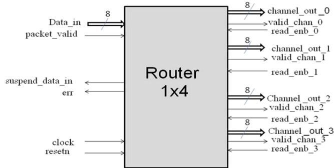
Figure 1: Block Diagram of Five Port Router
