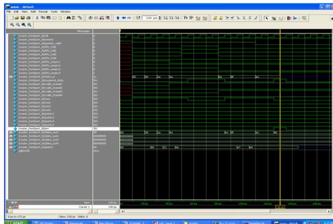
Figure 3: Simulation of FSM Controller
