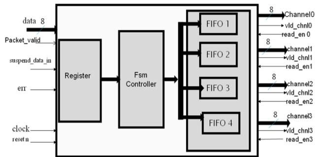
Figure 2: Internal Structure of Five Port Router
